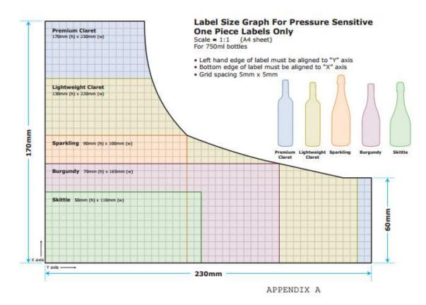
The Label Panel Chart shows the five most popular 750ml bottle styles (Premium Claret, Lightweight Claret, Sparkling, Burgundy and Skittle). The label should fit into the dimensions shown in the Label Panel Chart. The minimum label height is 12mm.
