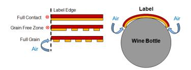
Lift may propagate more significantly if other factors are present (such as reduced contact area, label stiffness, etc.). Significantly, adhesive decay with a full grain may happen over time - and may not reveal itself for months or years.
