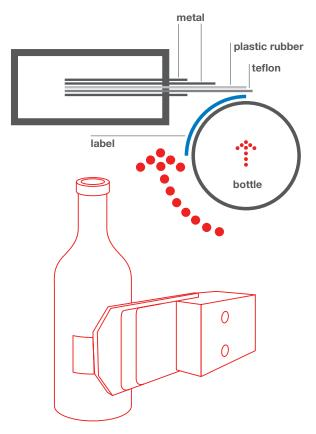
The automatic application process for pressure-sensitive labels dispenses a label from the release liner at a set point, brings
